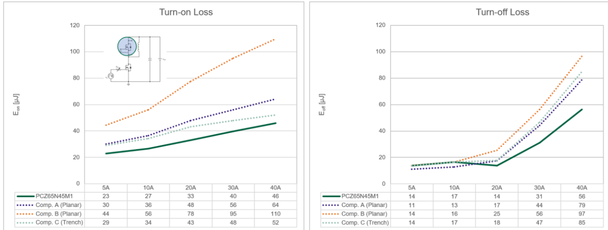
Figure 11. Comparison of Switching Losses - 650V/45m \Omega e -SiC MOSFET M1(PCZ65N45M1) vs. competitors under V_{DD}=400V , V_{GS}=-3V/+18V , R_G=2.7\Omega , Free-wheeling Diode: Same DUT
